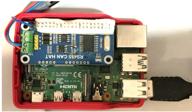
Fig. 2 The Raspberry PI 4B evaluation board with the power flow controller used as the main control for the system.
