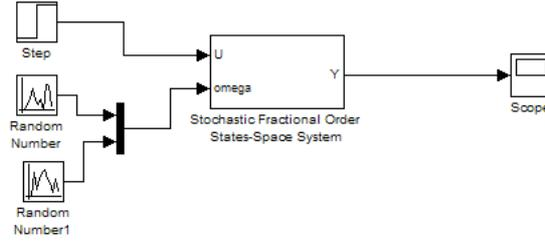
Figure 1: Using of the Discrete Stochastic Fractional Order State-Space System Block scheme
