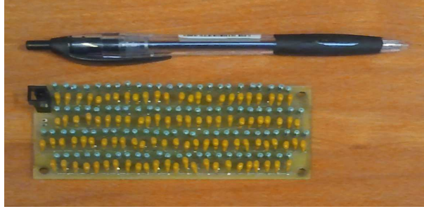
Fig. 1.4. A circuit board of 0.5 order impedance.
