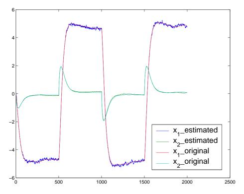
Figure 5: Results of states estimation in close-loop feedback control
